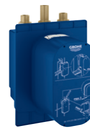
36 459 000 Concealed body for shower with transformer 100 – 240 V AC and integrated thermostatic mixer suitable for infra-red set 36 456 000
