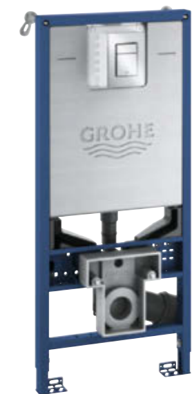
39 603 000 Rapid SLX WC 3-6 | 1.13 m with wall brackets and Skate Cosmopolitan S Chrome Rapid SLX Element for WC, 1.13 m installation height with flushing cistern GD2, with electric socket, including flow manager, easy access and fully insulated against condensation. With wall brackets and Skate Cosmopolitan S (chrome) flush plate.
