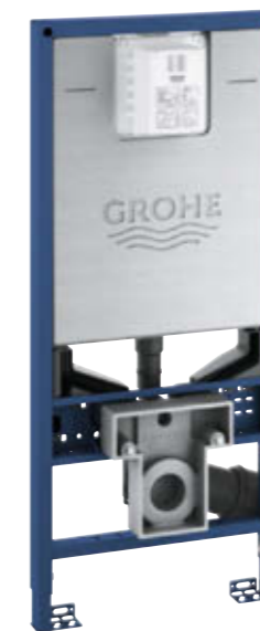
39 599 000 Rapid SLX WC 3-6 | 1.13 m F with heavy load feet Rapid SLX Element for WC, 1.13 m installation height with flushing cistern GD2, with electric socket, including flow manager, easy access and fully insulated against condensation. With heavy load feet.
