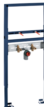
39 052 000 Rapid SL for wash basin height adjustable, for single hole installation, 1.13 m installation height, for on-the-wall installations or studded walls, 2 noise protected fitting connections 1/2"
