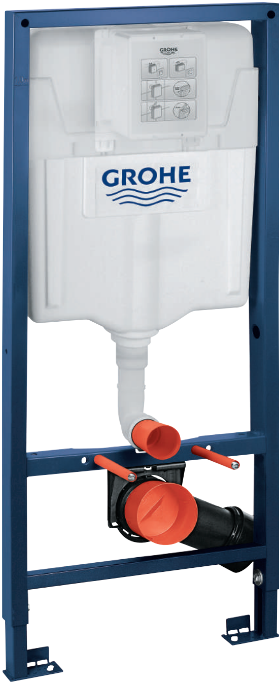
38 528 001 Rapid SL for WC with flushing cistern 6 – 9 l dual flush/start & stop/single flush connection from left/right/rear 1.13 m installation height
